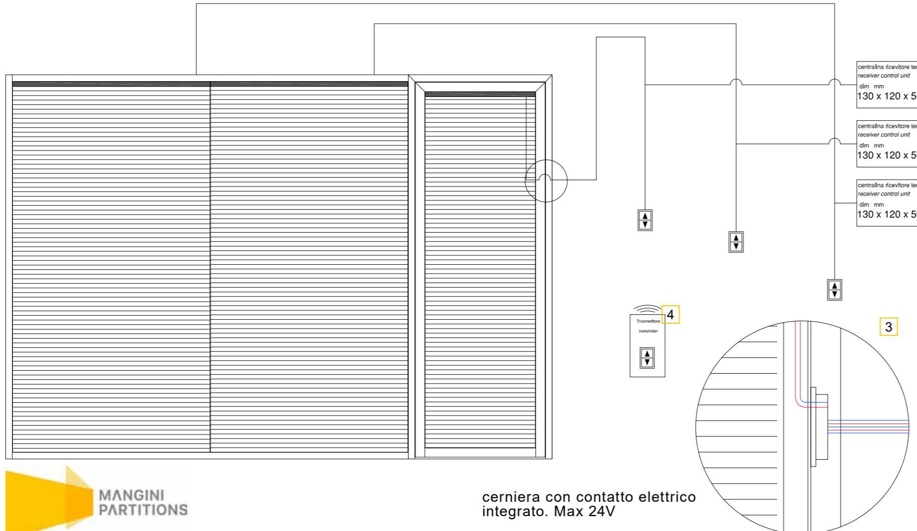
Flux ONE system provides for the possibility of inserting different types of motorized blinds between the panels in strips or in pleated fabric, filtering or completely blackout.
